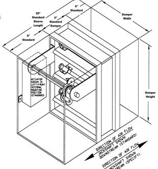
U.L. 555S Classified at 250°F or 350°F depending upon Motor/Operator \*See Motor/Operator Schedule
