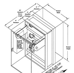
U.L. 555S Classified at 250°F or 350°F depending upon Motor/Operator \*See Motor/Operator Schedule
